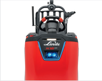
Linde BlueSpot™ and front LED light
