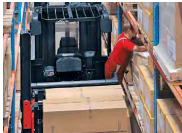
Order picking barrier: Tilting barrier for better access to cases at the back of a pallet optimising picking reach by approximately 50 cm
