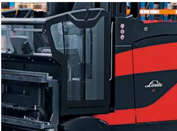
Glass door: Comfortable working environment due to wind and drafts being deflected
