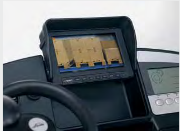
Video Camera: Best vision for pallet storage and retrieval at height
